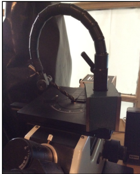
Figure 3. Viewing and measuring of drill tool flank wears by trinocular microscope.
