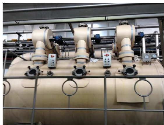
Figure 4. Dyeing machines isolated with highly cross-linked polyethylene foam manufactured insulation material
