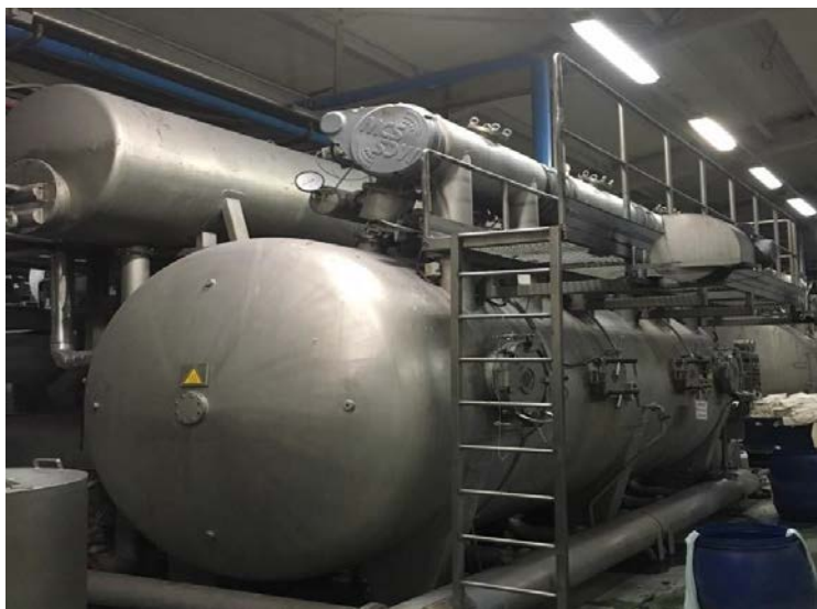
Figure 2. Dyeing machines without isolation
