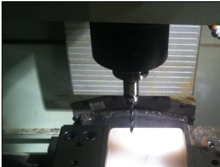
Figure 1. Drilling operation with HSS twist drill tool using CNC machining center.
