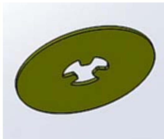
Figure 3. The schematic of the bimetal disc was die cutted for transducers
