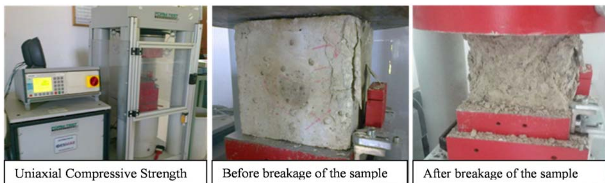
Fig. 3 Applying Uniaxial Compressive Strength Test on samples (Sabbag and Uyanık, 2015)
