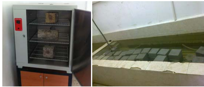
Fig. 4 Drying in an oven and applying water cure of the samples for the determination of water content
