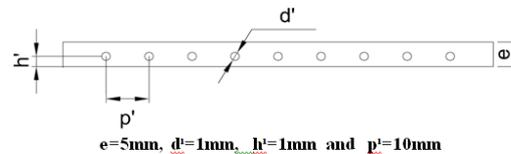
Figure 2: Schematic view of present perforated ribs
