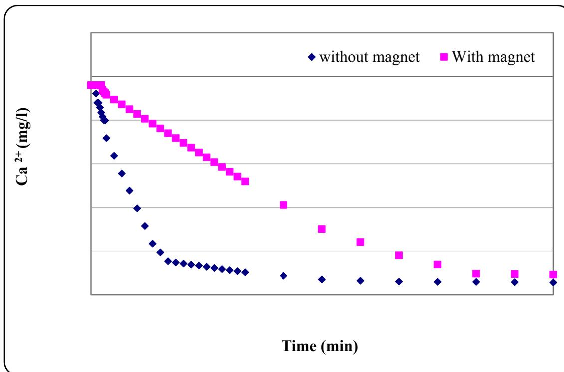
**Fig. 3.** Calcium ion analysis of CaCO<sub>3</sub> solution in flowing condition versus time.
