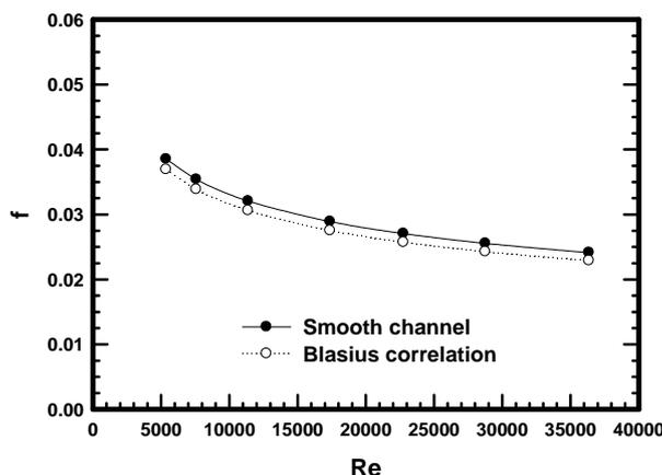
**Figure 4:** Verification of friction factor for smooth channel
