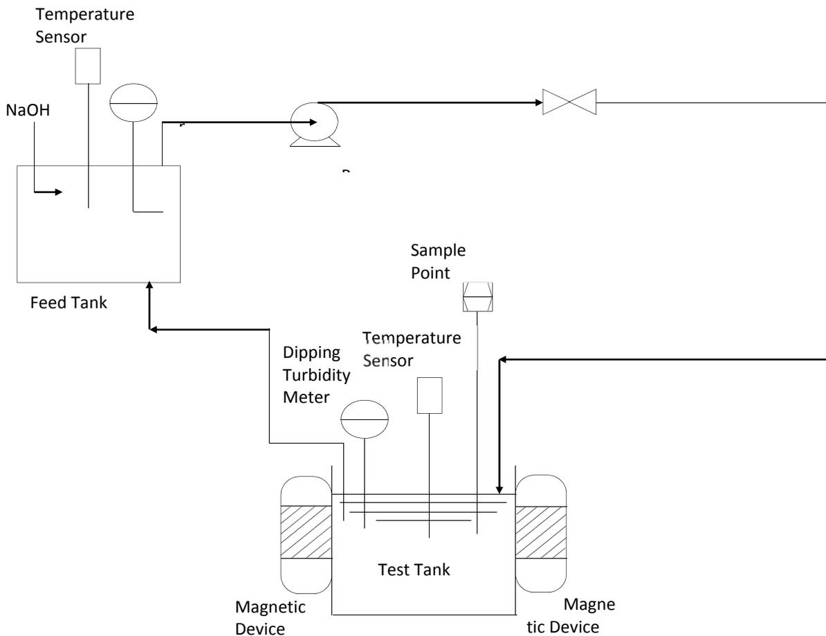
Fig. 1. The schematic of the experimental test plant.
