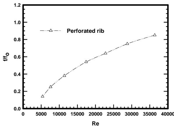
**Figure 7:** Friction factor ratio with Reynolds number
