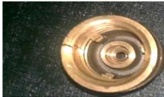
Fig. 11. Hot crack propagation in machined leaded brass
