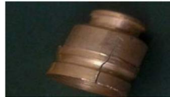
Fig. 12. Jaws marking and cracks in lead brass
