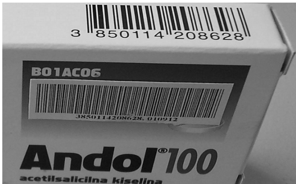
Picture 2. Sample of drug with extended barcode (front side) and EAN13 (top side)
