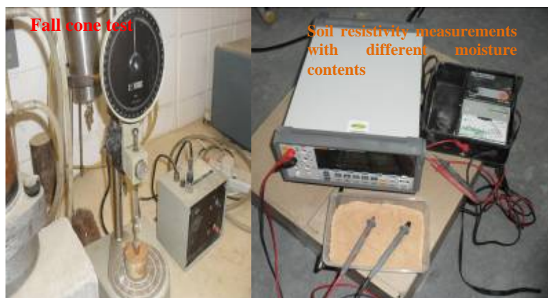
Figure 1. Soil electrical resistivity measurement for soil state determination
