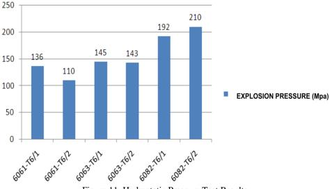
Figure 11. Hydrostatic Pressure Test Results
