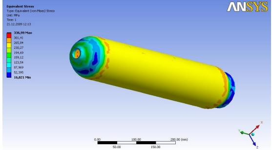
Figure 9. 6082 T6 201 Bar ANSYS Equivalent Stress Results
