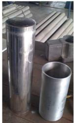
Figure 4. The comparison between first forming process and second forming process
