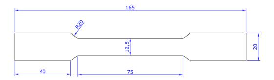
Figure 7. Dimensions of the tensile test samples coming out from the pipe according to TS 138 EN 10002-1 Graphs generated according to tensile test results are shown in Figure 8.
