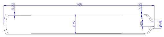
Figure 6. Tank Dimensions
