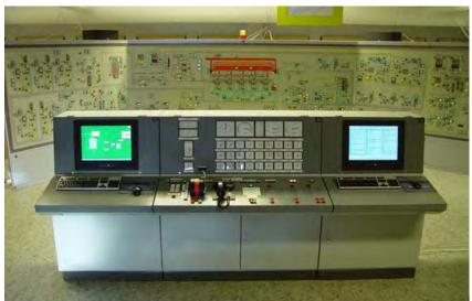
Fig. 2 General view of Engine Room Simulator (Kongsberg, 2008)
