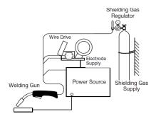
Fig. 3: Gas Metal Arc Welding
