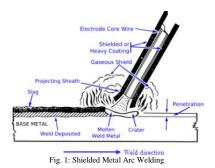
This welding method is used for maintenance and repair industries, naval industry, pipelines, offshore platforms, construction of steel structures, weld carbon steel, low and high alloy steel, stainless steels, cast iron, aluminum, nickel and cooper alloys.
