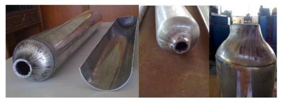
Figure 5. Shrinking process for end part of the Aluminum-hydrogen tank
