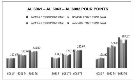
Figure 8. Pour Point Results Of Al 6061-Al 6063-Al 6082 Alloys Obtained By Tensile Tests
