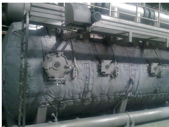
Figure 3. Dyeing machines isolated with silicone coated glass fiber and glass wool blended material
