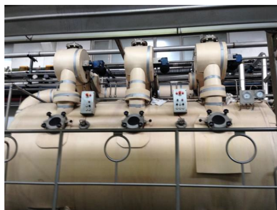
Figure 4. Dyeing machines isolated with highly cross-linked polyethylene foam manufactured insulation material
