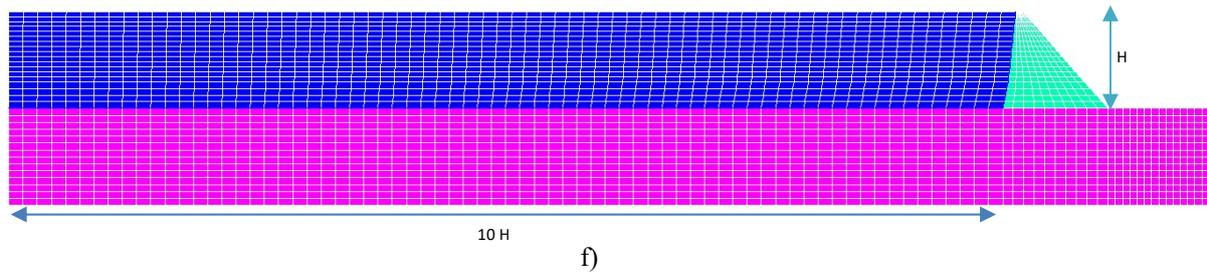
**Fig. 2.** Finite Element Models of Cine RCC dam
