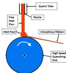
**Figure 1.** Schematic view of melt spin apparatus (Wang& Mitra, 2014)
