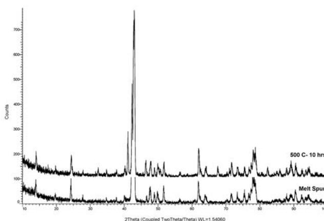
**Figure 2.** XRD of melt spun and heat treated at 500°C for 10 hrs melt spun ribbons.
