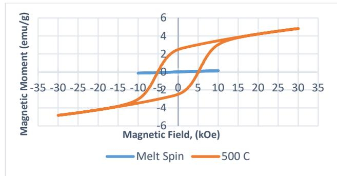
**Figure 3.** Magnetic hysteresis of Melt spin and heat treated at 500°C for 10 hrs melt spun ribbons at 305 K
