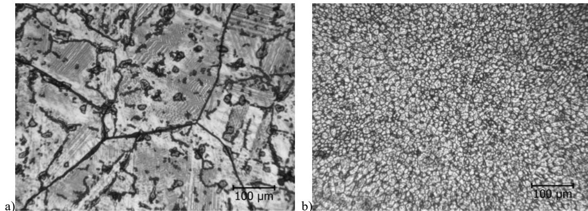
**Figure 4.** a) Cast and heat treated sample, b) melt spun and heat treated sample, both heat treated at 500°C for 10 hrs
