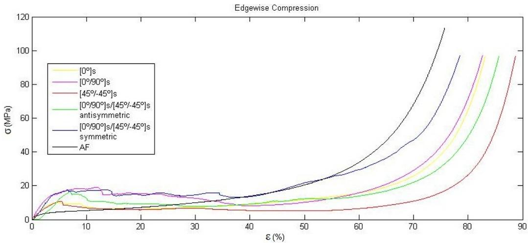
**Figure 4.** Stress-strain curves measured under static edgewise compression
