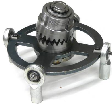
Figure 4: Swing plate with rod ends and gear
