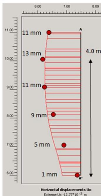
Figure 3.1 Horizontal deflection of the wall
