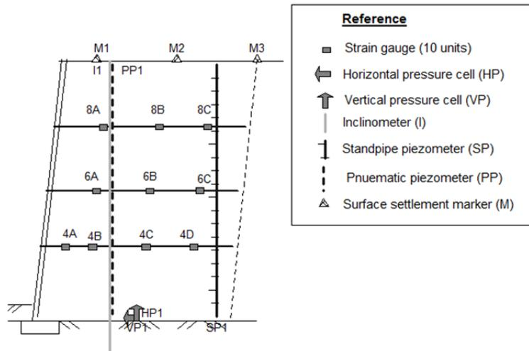
**Figure 2.2** Location of various type of instrument
