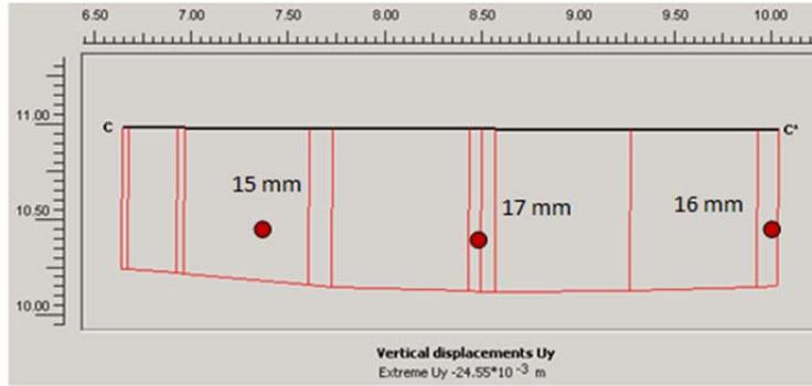
Figure 3.2 Surface settlement of the wall
