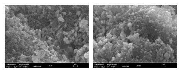
Figure 3. SEM microstructures of 28 day water cured A and D series samples.
